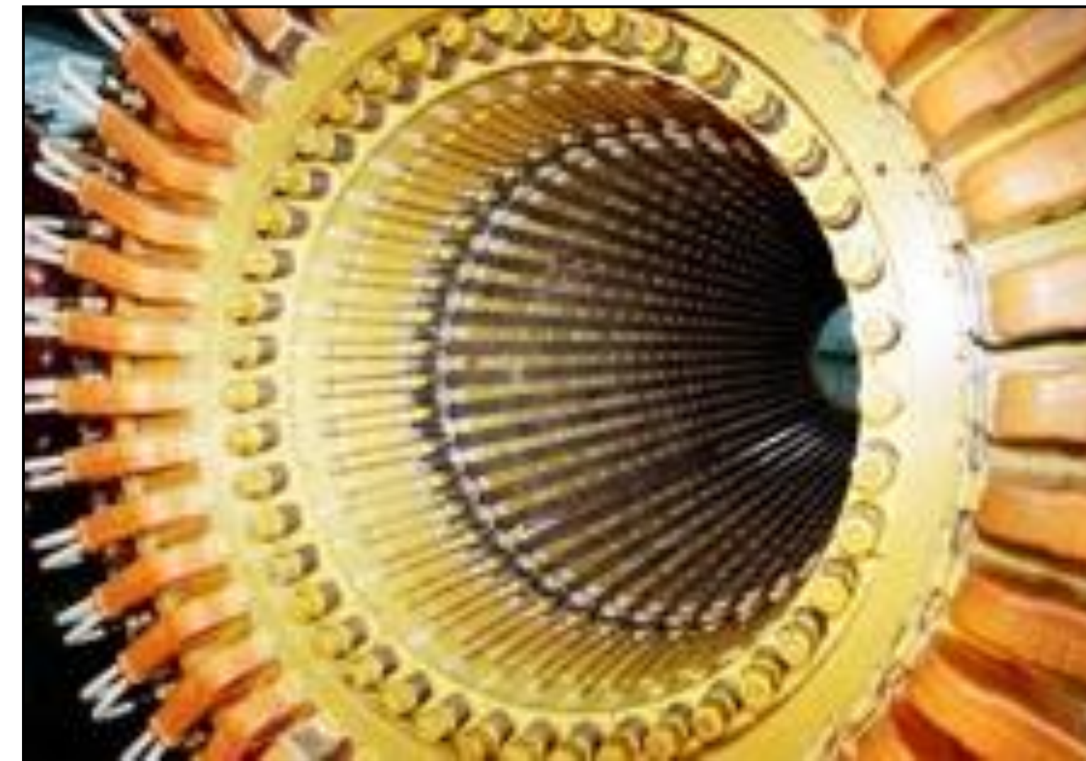
Fig. 1. The end part of power turbine generator stator. 1 – stator winding; 2 – pressure plate; 3 –electromagnetic shield; 4 – pressure fingers; 5, 6 – stator core packets
