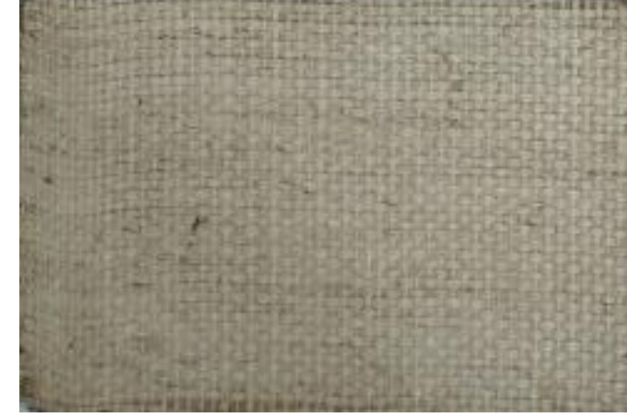
Figure 6. Fique fiber laminate with unsaturated polyester resin.
