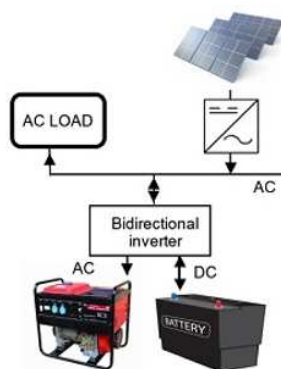
Fig. 1. Off-grid PV-Diesel-battery system.
