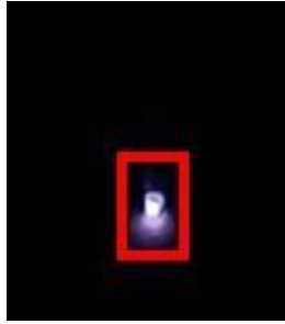
Fig. 3. Long-exposure image of a corona discharge on the tip of the needle-plane electrode taken with the BI-CMOS sensor.
