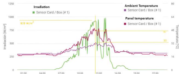
Fig. 11. Effect of ambient temperature and radiation on panel temperature.
