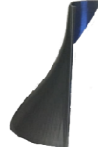
Fig. 3. Real-scale 3D printed blade model.
