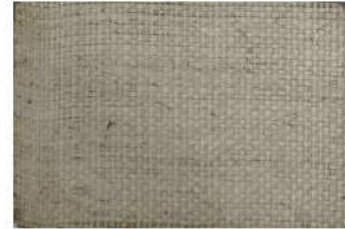
Fig. 1. Fique fiber laminate with unsaturated polyester resin
