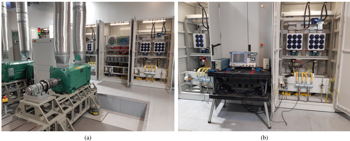
Fig. 8. Measurement setup in the laboratory. (a) Location of the DAB converter, (b) probe arrangement.
