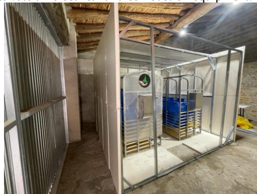
Fig.2. Thermally insulated enclosure where the digesters are located.
