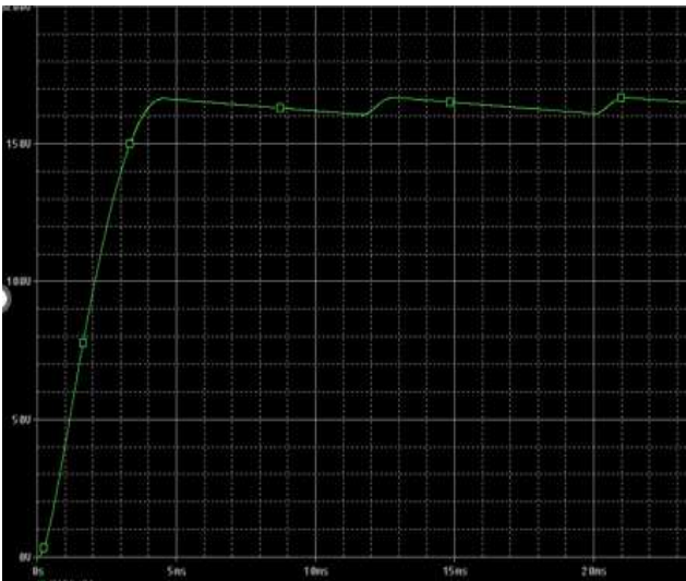
Figure 2: Output Voltage of the FWBR with Capacitor
