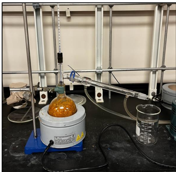
Fig. 4 Steam distillation setup. A 500 ml round-bottom flask contained the solution, while a thermometer and tube were attached to the top for distillation to occur and be monitored.
