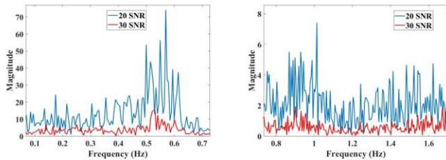
Fig. 3. Frequency spectrum of  $P_g$  of synchronous generator G4 for Cases 1 and 3
