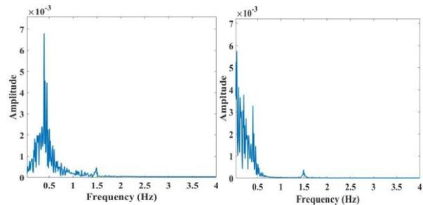
Fig. 9. Frequency spectrum of  $P_g$  of synchronous generator at bus 1 and 2 for DFIG at Bus 3
