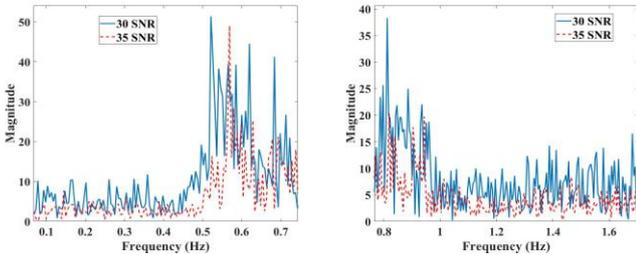
Fig. 4. Frequency spectrum of  $P_g$  of synchronous generator G4 for Cases 2 and 4
