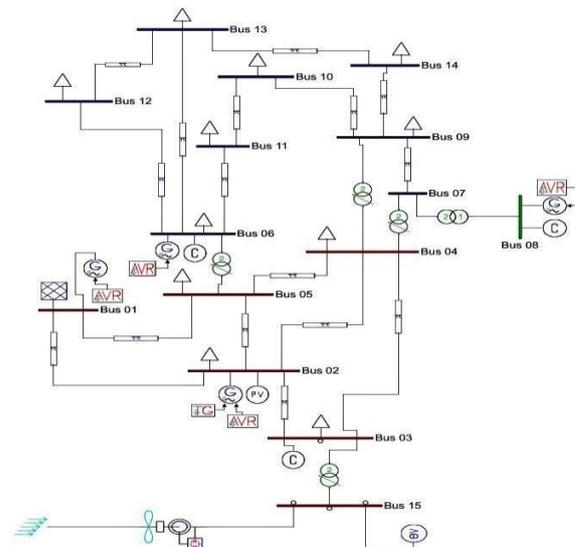
Fig. 5. Modified IEEE 14 Bus system with DFIG at Bus 3
