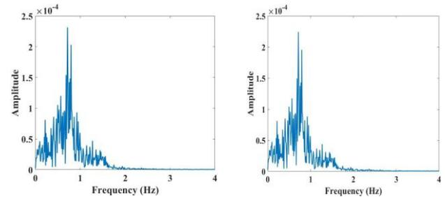
Fig. 8. Frequency spectrum of  $P_g$  of synchronous generator at bus 8 and 6 for DFIG at Bus 1
