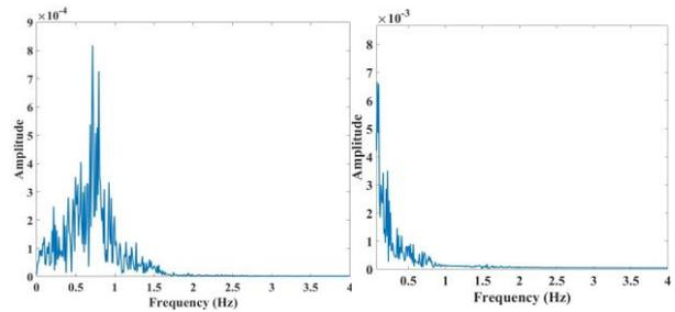
Fig. 7. Frequency spectrum of  $P_g$  of synchronous generators at bus 3 and 2 for DFIG at Bus 1
