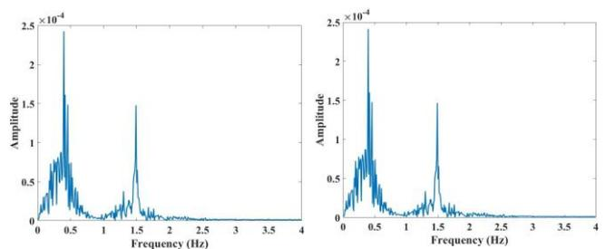
Fig. 10. Frequency spectrum of  $P_g$  of synchronous generator at bus 8 and 6 for DFIG at Bus 3
