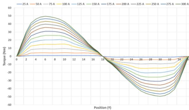
Fig.7. Static torque curves of the final SSSRM design
