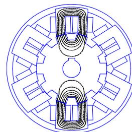
Fig. 1. Cross-section of a 12/10 SSSRM showing the distribution of the magnetic field lines.
