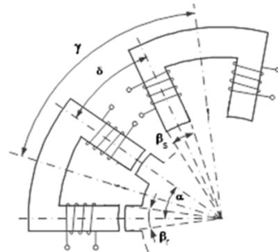
Fig. 4. Basic arrangement of an SSSRM.
