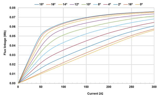
Fig. 6. Magnetization curves of the final SSSRM design.
