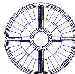
Fig. 2. Distribution of the magnetic field lines in a 12/8 SRM
