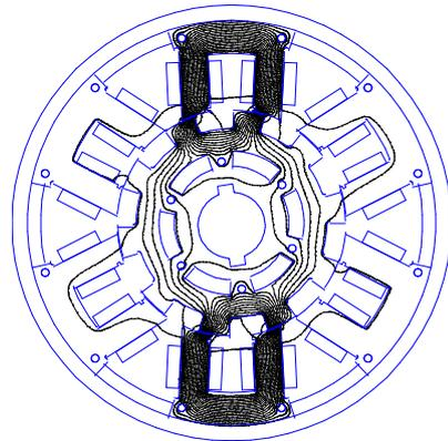
Fig. 5. Distribution of magnetic flux field lines for a position  $9^\circ$  from unalignment in the SSSRM.
