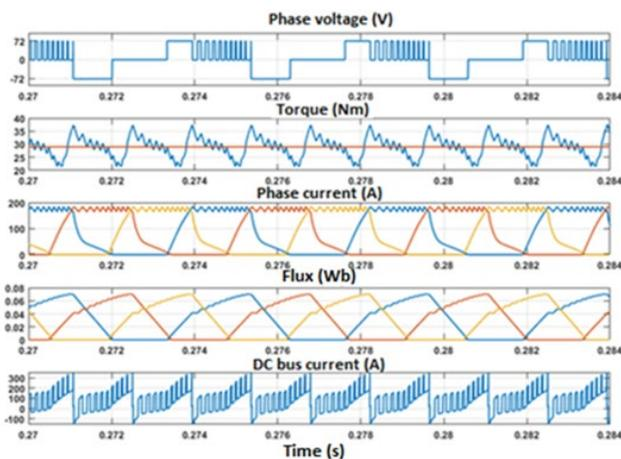
Fig. 8. Simulated values of phase voltage, torque, phase current, flux and dc bus current for a torque of 28 Nm at 1400 rpm.
