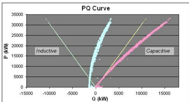
Fig. 2. PQ curve and requirements stipulated by RD 436/2004
