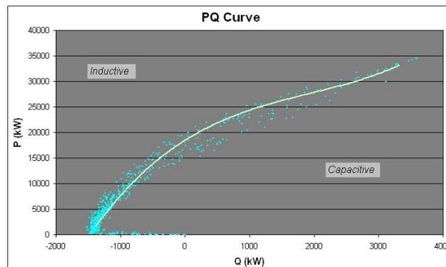
Fig. 3. Description of PQ curve at the Munilla wind farm
