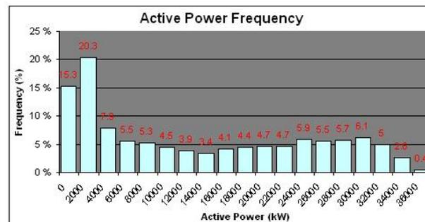
Fig. 4. Active Power Frequency generated by wind farm
