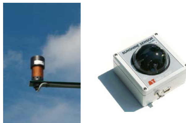
Fig. 2 – Wind speed and solar radiation sensors.
