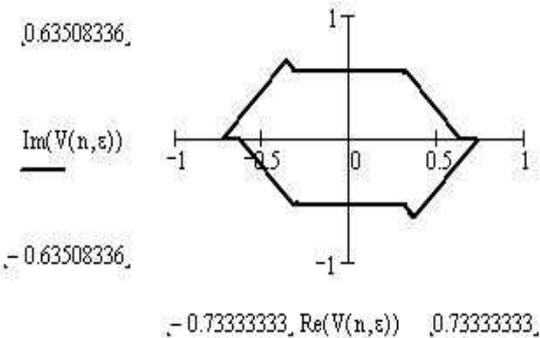
Fig.4-Trajectory of overall stator voltage vector
