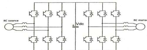
Fig.1. Basic scheme of VSI with AC motor
