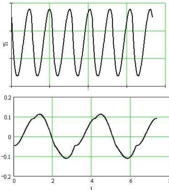
Fig.12. Electromagnetic torque waveforms. Top – without any DC link components. Bottom -Contribution from DC link ripple.
