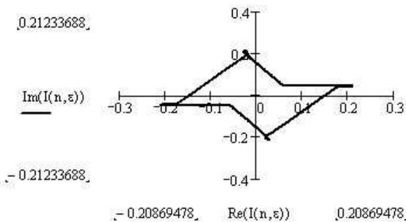
Fig.7 Overall stator current trajectory in complex plane
