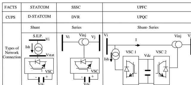
Fig. 3. Connected DFACTS devices
