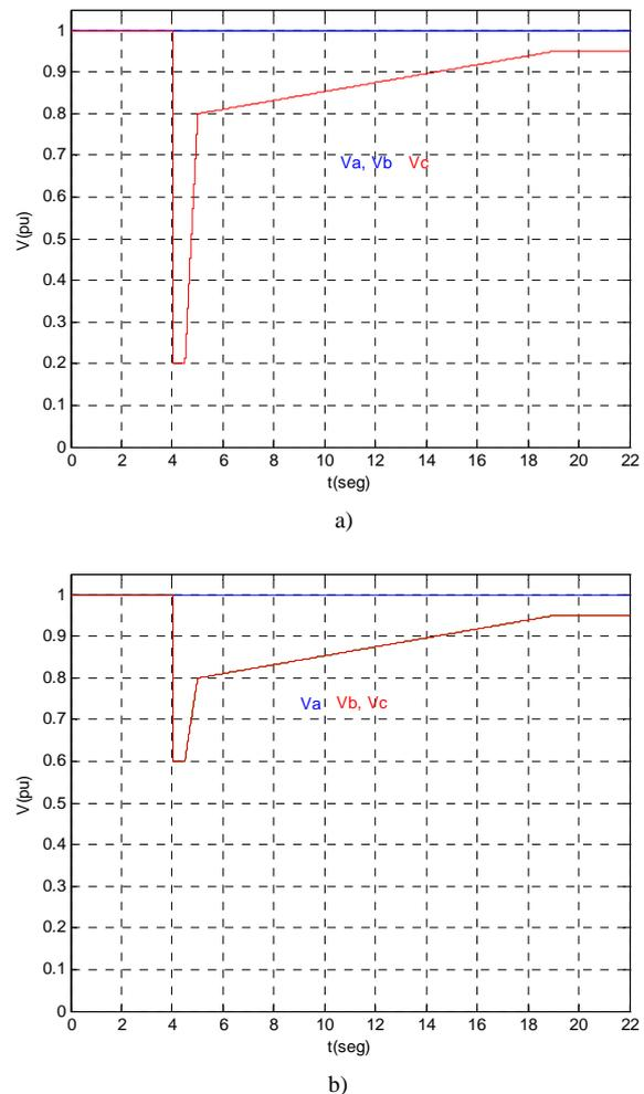
Fig. 4. Voltage-Time curve a) One-phase dip b) two-phase dip
