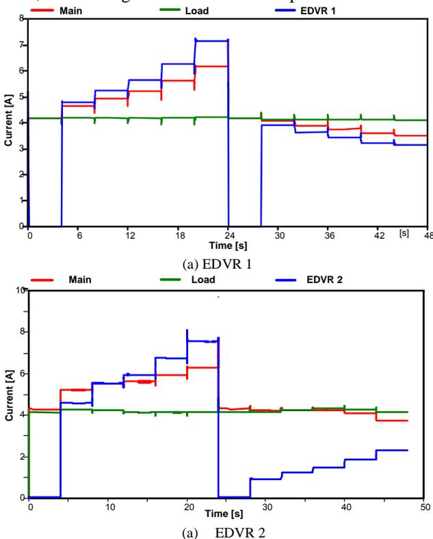
Fig. 11. Currents at the supply, load and compensators: (a) EDVR 1 (b) EDVR 2.
