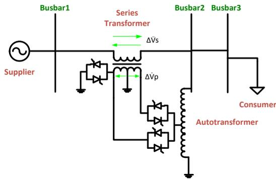
Fig. 5. Continuous voltage compensator conception – Proposal 2 (EDVR 2)
