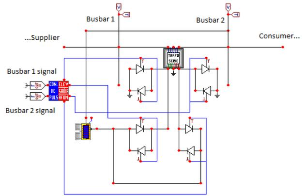
Fig. 7. The electromagnetic voltage regulator model - ATPDraw Platform - EDVR 2
