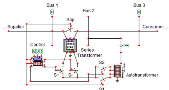
Fig. 4. The electromagnetic voltage regulator model - ATPDraw Platform - EDVR 1
