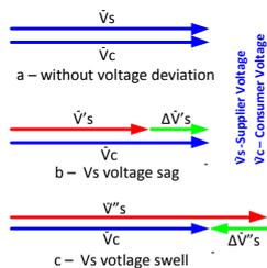
Fig. 2. The device voltage compensation principle
