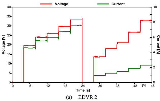
Fig. 10. Voltage and current at EDVR 1 - (a) and EDVR 2 - (b) - values at the autotransformer secondary and series transformer primary side
