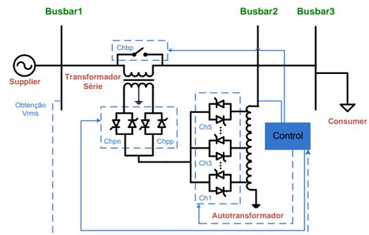
Fig. 3. Discrete tap changer physical structure conception – Proposal 1 (EDVR 1)
