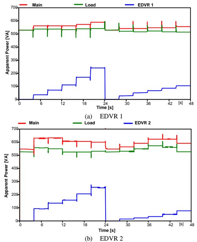
Fig. 12. Apparent power at the mains, load and compensators: (a) EDVR 1 (b) EDVR 2.
