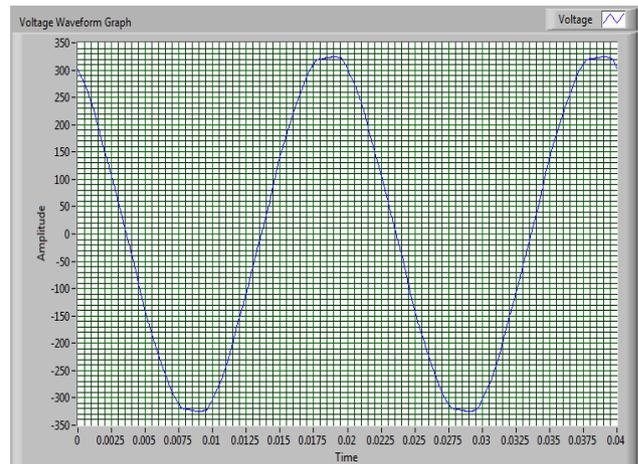
Fig. 5. Voltage waveform graphs of ECO Energy saving light,  $THD_V=1,57\%$
