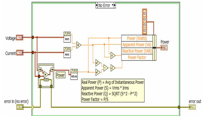
Fig.2 Block diagram-source code of the subroutine POWER
