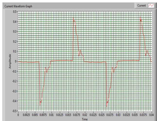
Fig. 6. Current waveform graphs of ECO Energy saving light,  $THD_I=113,12\%$
