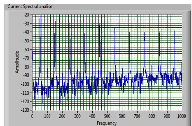
Fig. 7. Current spectral analysis for ECO Energy saving light
