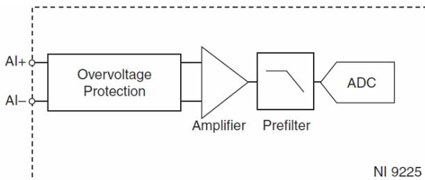
Fig. 1. Input circuits for one channel of NI voltage analogue input module
