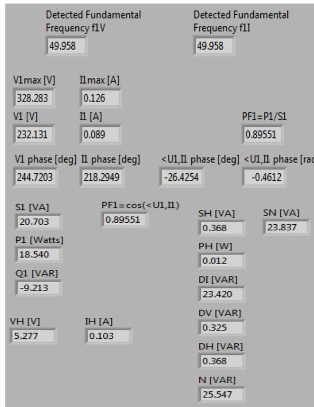
Fig. 8. Power measurements according IEEE Std. 1459 for ECO Energy saving light
