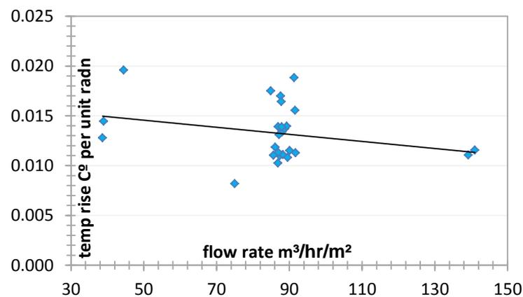
Fig.8 Variation of temperature rise per unit radiation against flow rates.
