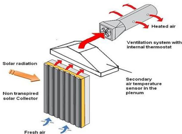
Fig.4. BPSC system schematic
