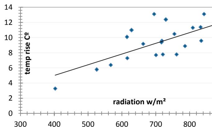
Fig.7 Variation of temperature rise against radiation for middle air flow rates.
