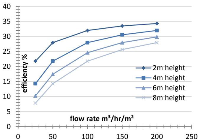
Fig.9 Variation of percentage efficiency against flow rate
