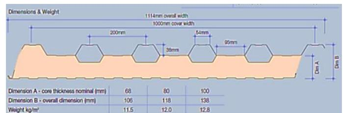
Fig. 2. BPSC cross section and measures
