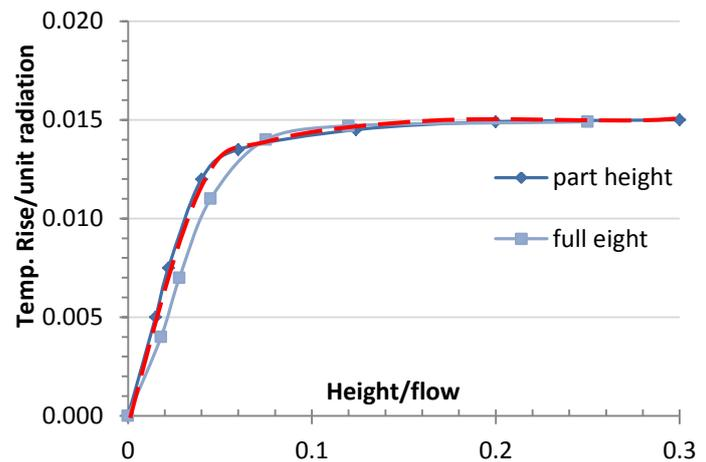
Fig.10 Variation of temperature rise per unit radiation against flow rates
