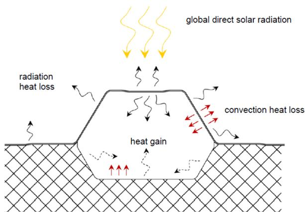
Fig.3. BPSC energy flow section.
