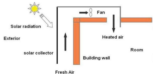
Fig. 1. Solar air collector system schematic
