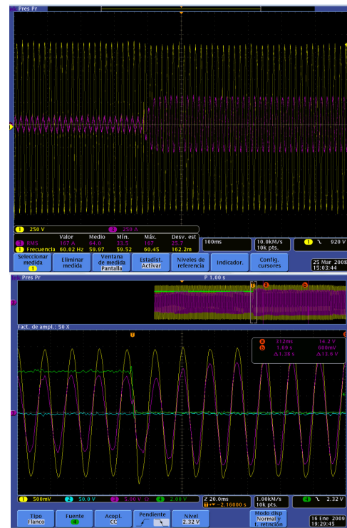
Fig. 6 Oscilloscope results showing voltage and current responses to load changes
