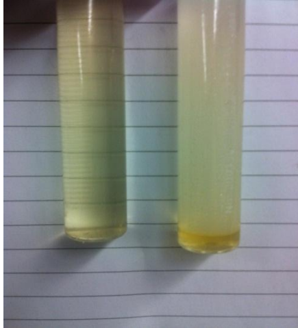
Fig. 3 - A passed 27/3 test using ultrasonication (left) and a failed test using conventional stirring (right).
