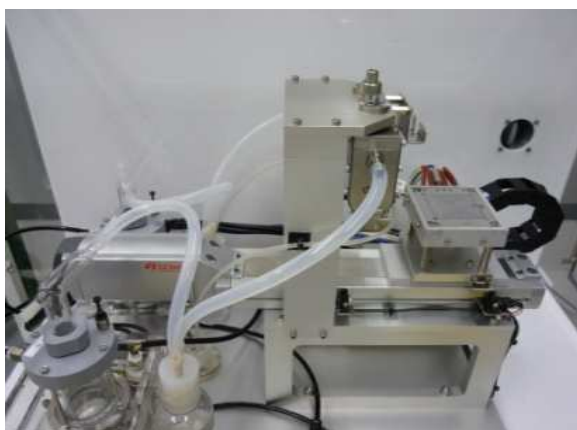
Fig. 1 Schematic illustration of the modified spray-mist coating process (above) and a picture of the apparatus (bottom). The donor (P3HT) and acceptor (PCBM) solutions are atomized in two separate mist sources as fine channel mist spray deposition (FCMSD).
