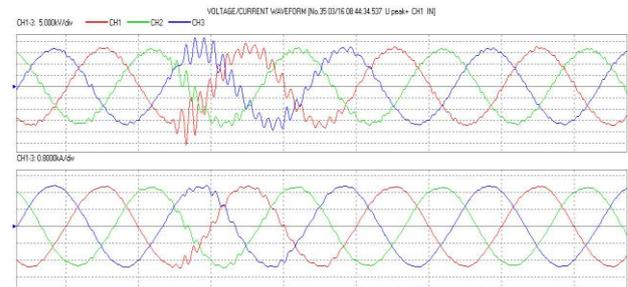
Fig. 8. Voltages and currents at 20kV, after modifications in the wind turbines
