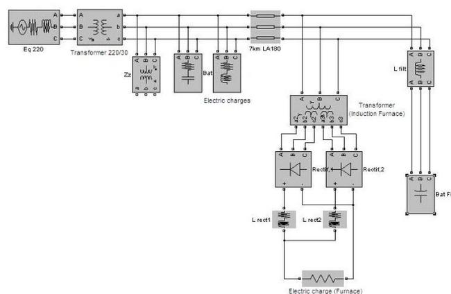
Fig. 1. Simplified diagram of the facility
