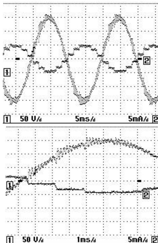
Fig. 2. Induction furnace current and effect on voltage
