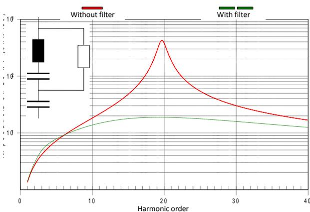
Fig. 7. Effect of damped filter on cable resonance
