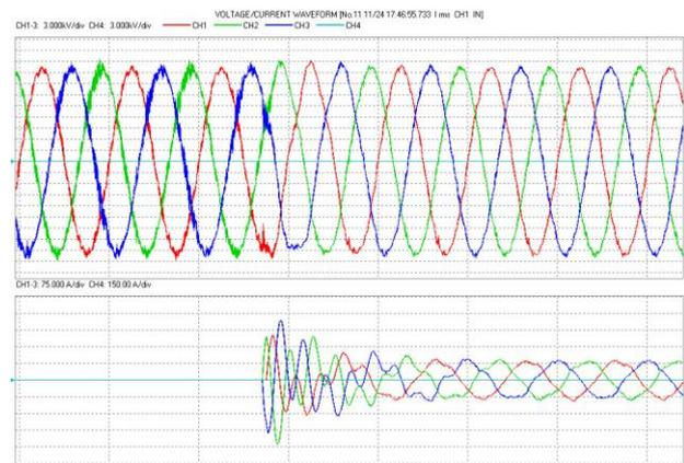
Fig. 4. Filter connection and elimination of the disturbance
