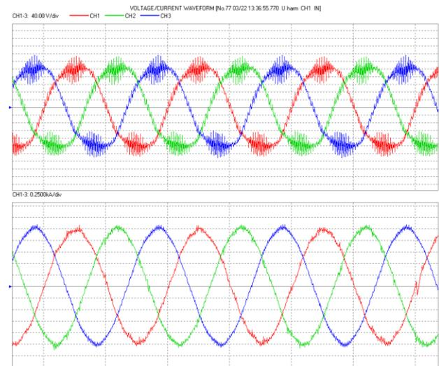
Fig. 8. Voltage and current distortion in normal operation of LV photovoltaic generator
