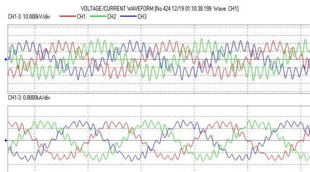
Fig. 6. Voltages and currents at 20kV, with incidents in wind turbines
