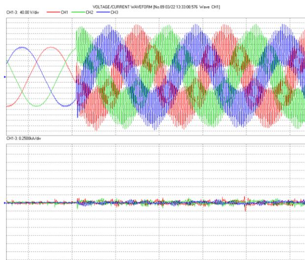
Fig. 9. Voltage and current distortion during synchronization of LV photovoltaic generator
