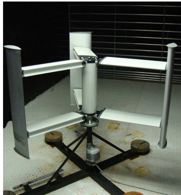
Figure 1: Image of the Ropatec (150W) [6] wind turbine used in this study.
