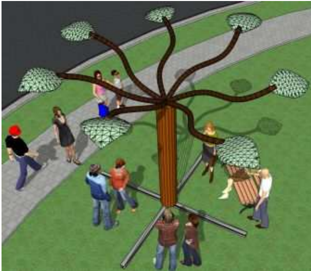
Figure 1: Concept drawing of the solar tree, showing the wooden stem, iron roots and the photovoltaic cells on top of the leaves.
