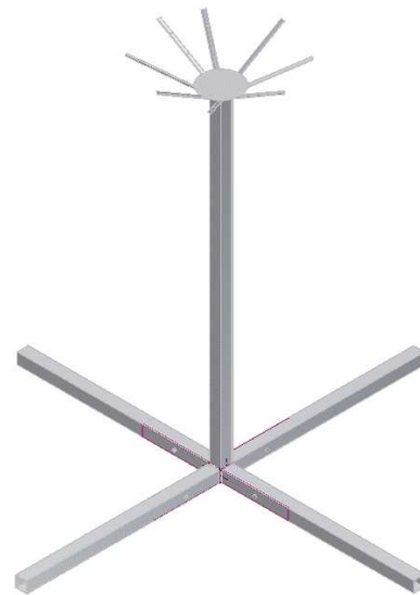
Figure 2: The iron welded skeleton of the tree, containing rectangular iron profiles with 120 mm in diameter and a thickness of 5 mm
