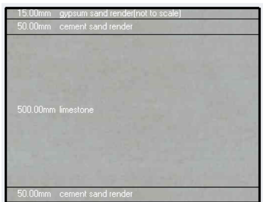
Figure 2 – Wall layers (3rd floor) DesignBuilder figure
