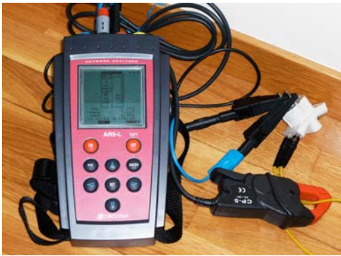
Fig. 2. Power network analyzer AR5-L of CIRCUTOR.
