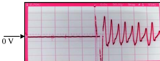
Fig.8. For a 200W/phase lamp load the phase 'a' current with prime mover speed of 1440 rpm
