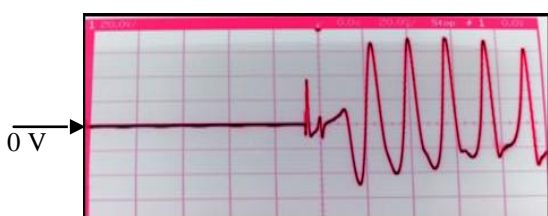
Fig.9. Voltage build up at a prime mover speed of 1750 rpm
