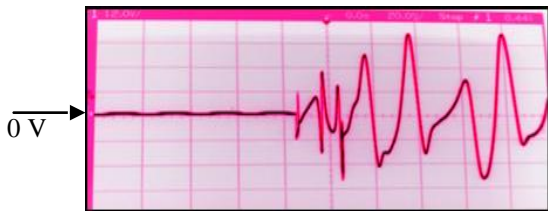
Fig.7. The voltage build up process for a prime mover speed of 1440 rpm
