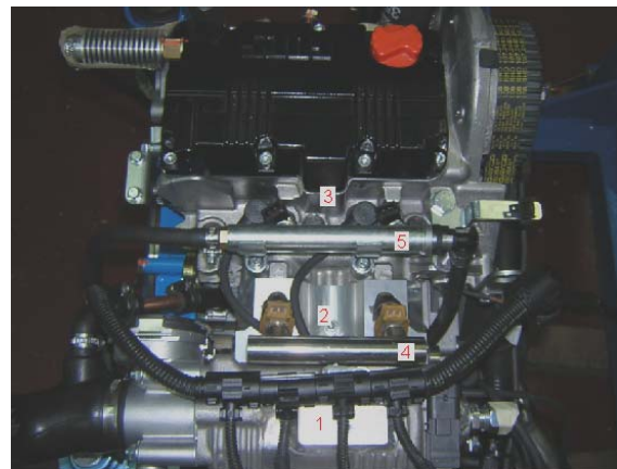
Fig. 1. Some modifications made in the inlet manifold. (1-Air inlet manifold; 2-Secondary manifold; 3-Cylinder head; 4-Gaseous fuel injection system; 5-Gasoline fuel injection system)
