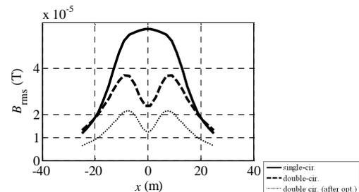
Fig. 1. Magnetic field density calculations for single-circuit and double-circuit Slovenian overhead power lines.
