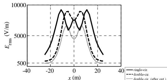
Fig. 2. Electric field strength calculations for single-circuit and double-circuit Slovenian overhead power lines.
