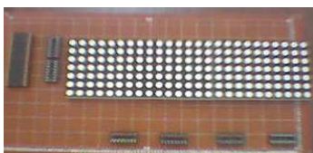
Fig. 9 IC Sockets and dot-matrices mounted on a stripboard.
