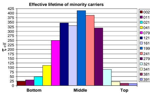
Figure 4: Evolution of the effective minority carrier lifetime along the ingot for n-type multicrystalline silicon samples, using  $\mu$ w-PCD technique.
