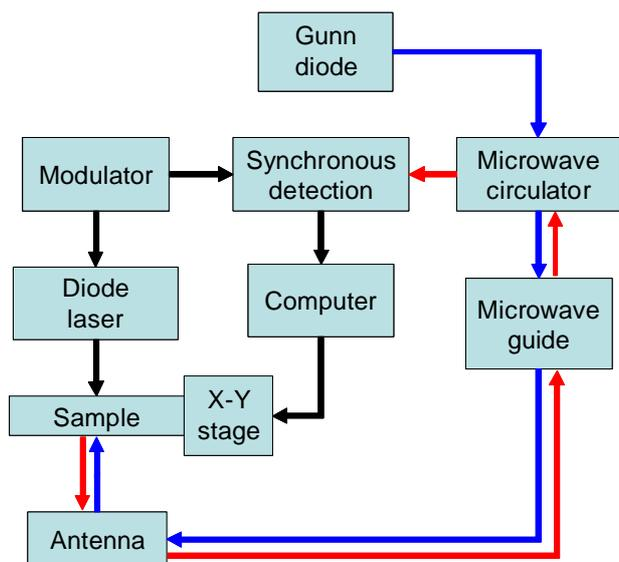
Figure 3: Schematic representation of the apparatus to lifetime measurements. The same set-up is used for  $\mu\text{w}$ -PCD and  $\mu\text{w}$ -PS techniques.
