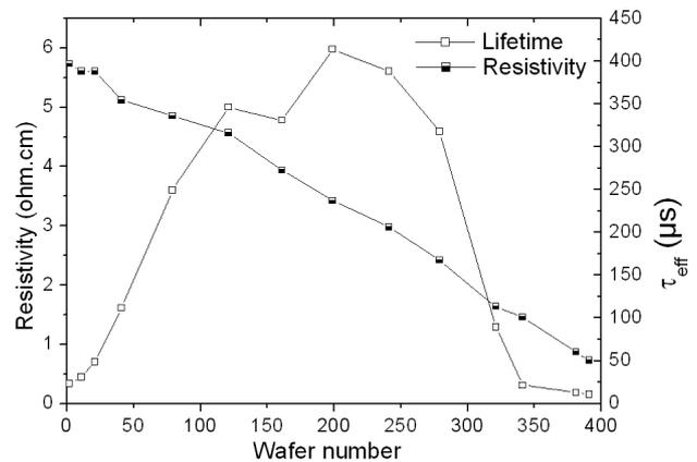
Figure 6: Resistivity profile and effective carrier lifetime evolution along the ingot height.
