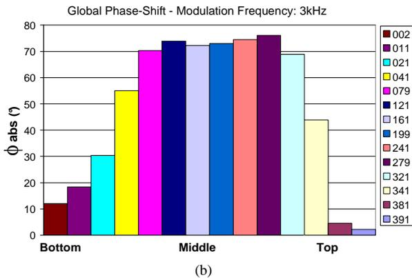
Figure 7: Evolution of the phase-shift along the n-type multicrystalline silicon ingot. (a)  $\mu$ w-PS technique and (b) LS- $\mu$ w-PS Technique.
