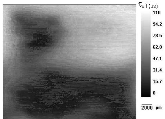
Figure 9: Scanning map over a compensated UMG silicon wafer. Both p-type and n-type are present side-by-side.
