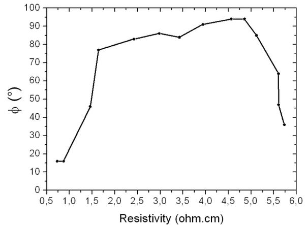
Figure 8: Phase-shift variation, obtained by  $\mu$ w-PS technique at 6 kHz, in function of resistivity profile at the ingot.
