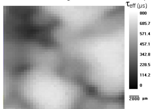
Figure 5: Effective carrier lifetime scanning maps (35mm x 35mm) in n-type multicrystalline EG silicon, obtained by  $\mu$ w-PCD technique.
