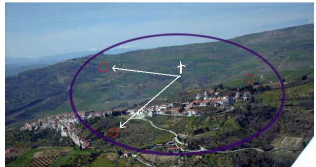
Fig. 5. Intervisibility analysis. The scheme underline the point in which is possible the see the wind farm (O) and ones in which isn't possible to see its.
