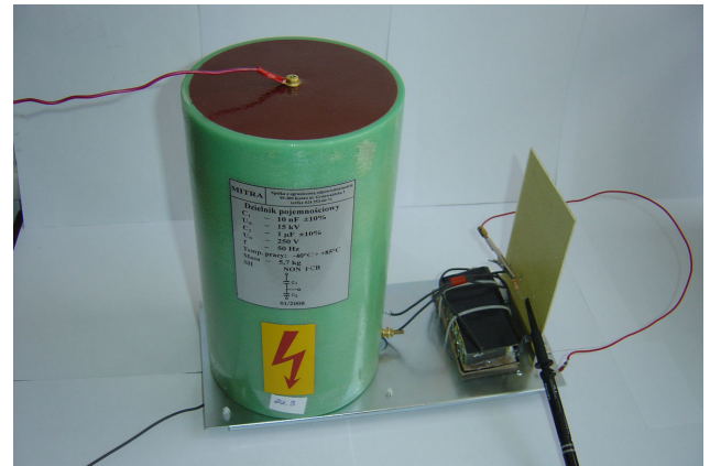
Fig. 11 A laboratory model of 10nF/1μF voltage divider
