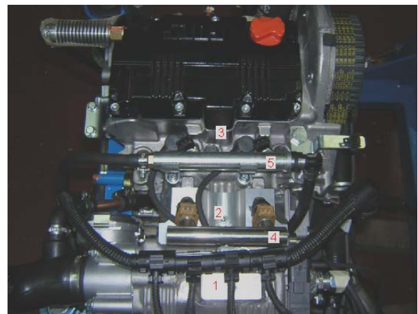
Fig. 2. Some modifications made in the inlet manifold. (1-Air inlet manifold; 2-Secondary manifold; 3-Cylinder head; 4- Gaseous fuel injection system; 5-Gasoline fuel injection system)
