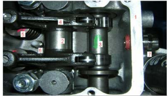
Fig. 3. Installation of cylinder head pressure sensor. (1-Cylinder head; 2-Rocker-arm shaft; 3-Camshaft; 4-Rocker arm; 5-Valve; 6-Combustion chamber pressure sensor; 7-Bulkhead)
