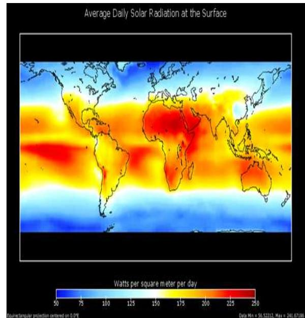
Fig. 4. The amount of solar radiation reaching the ground [11]
