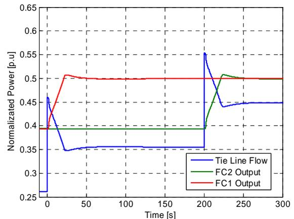
Fig. 11. Load Following performance of FC1, FC2, 50% increase of Load
