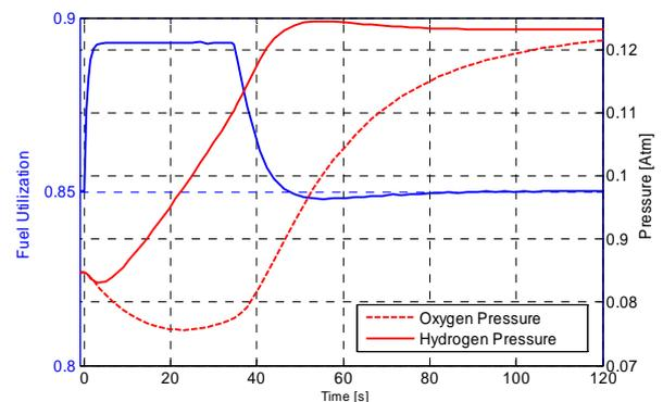
Fig. 4. Response of  $P_{H_2}, P_{O_2}$  and fuel utilization, to step in increase of power
