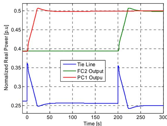
Fig. 7. Load-following performance of FC1, FC2, 25% increase of Load
