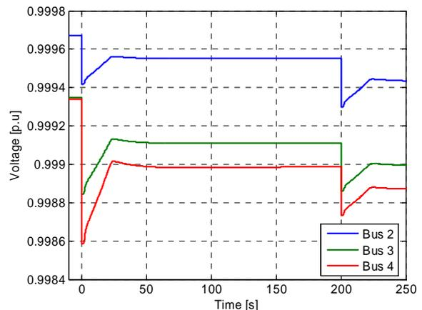
Fig. 13. Bus Voltage during 50% load change
