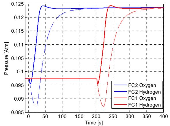
Fig. 10. Response of  $P_{H_2}$ ,  $P_{O_2}$ , for FC1 and FC2, 25% increase of Load
