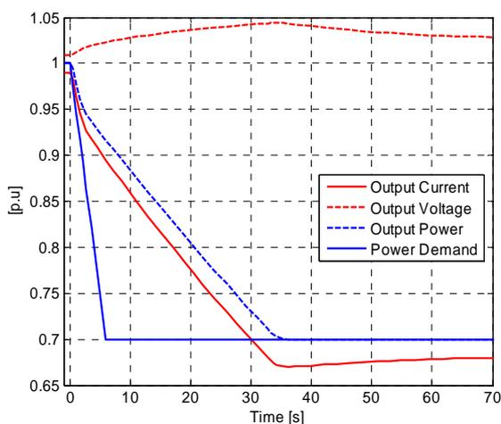
Fig. 5. Response of  $P_d$ ,  $P_{fc}$ ,  $V_{fc}$ ,  $I_{fc}$ , to ramp on decrease of power
