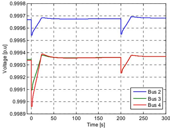
Fig. 8. Bus Voltage during 25% load change
