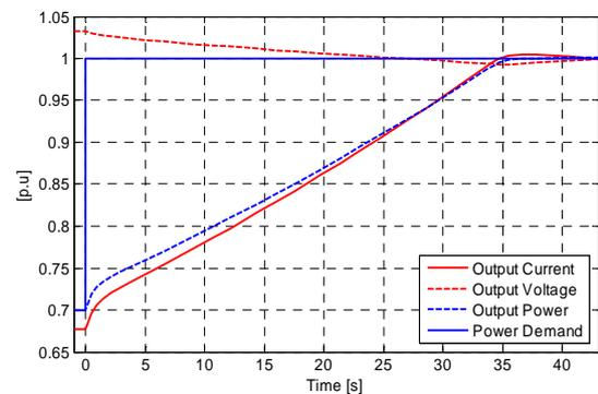
Fig. 3. Response of  $P_d, P_{fc}, V_{fc}, I_{fc}$ , to step in increase of power
