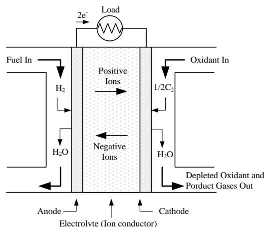
Fig. 1. Schematic of an Individual FC
