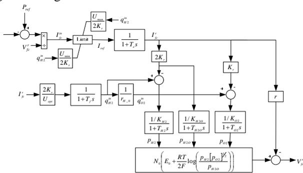
Fig. 2. SOFC system dynamic model
