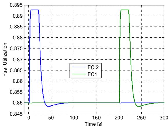
Fig. 9. Response of fuel utilization of FC1 and FC2, 25% increase of Load
