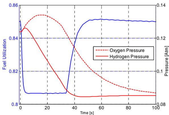
Fig. 6. Response of  $P_{H_2}$ ,  $P_{O_2}$  and fuel utilization, to ramp on decrease of power
