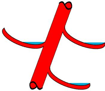
Figure 6. Contained mud in a screw section.
