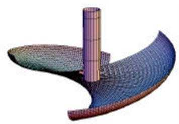
Figure 3. Double helix boot with semielliptic generatrix.
