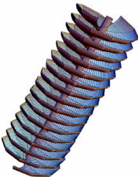
Figure 2. Double helix Arquimedes screw with semielliptic generatrix
