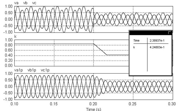
Fig. 9 – Three-phase PLL and Positive Sequence Detector during a 50% voltage sag.
