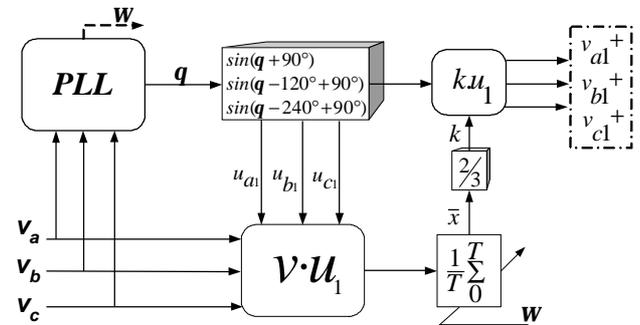
Fig. 4 – Algorithm of the Positive Sequence Detector.
