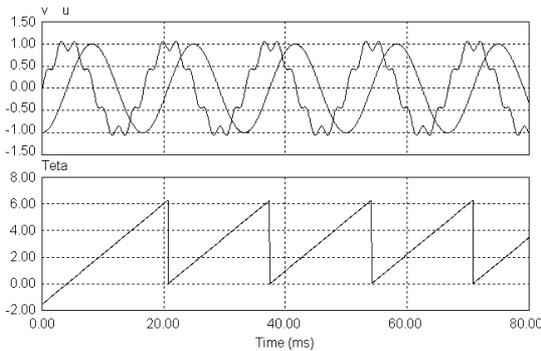
Fig. 5- Single-phase PLL: Distorted input voltage, PLL quadrature sinusoid and its argument angle  $\theta$ .
