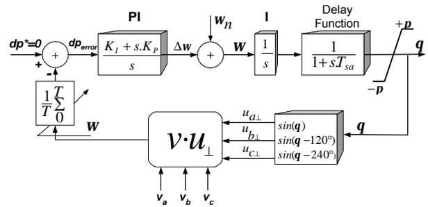
Fig. 3 - Three-phase digital PLL using instantaneous inner product of orthogonal functions.
