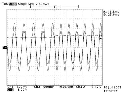
Fig. 11 – PLL action during a frequency step from 50 to 60Hz.
