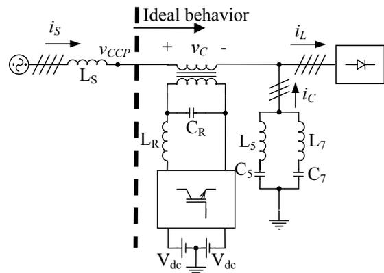
Fig. 1. Scheme of a hybrid filter, series active filter and shunt passive filter
