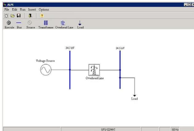
Fig. 3. ALPE – Basic 34.5kV Power System representation
