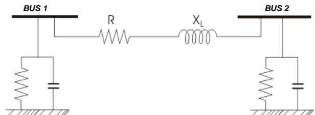
Fig. 1. Typical transmission/distribution line  $\pi$ -circuit representation
