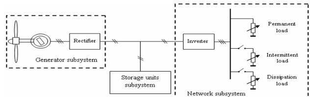
Fig. 1. Energy transfer subsystems
