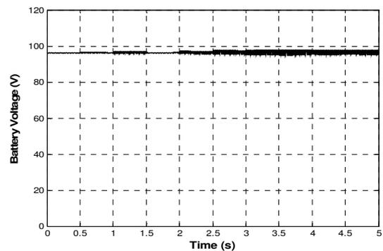
Fig. 5. Battery voltage evolution in buffer operating mode
