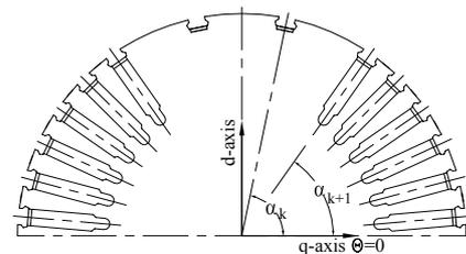
Fig. 3. Rotor cross-section with damper bar angular position
