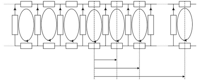
Fig. 2. Rotor damper winding impedance network
