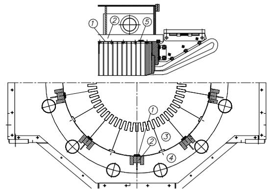
Fig. 4. Geometry of stator damper winding
