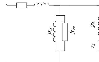
Fig. 5. Equivalent circuit of stator damper winding
