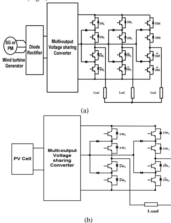
Fig.1. Using MOVS converters in renewable energy systems for (a) three-phase and (b) single phase applications with three-level diode-clamped inverter
