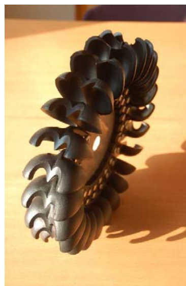
Fig. 5. The Pelton turbine
