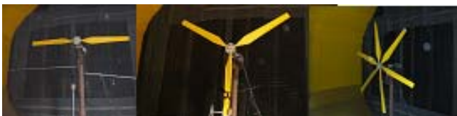
Fig. 2-Experimental rotors with type a blades
