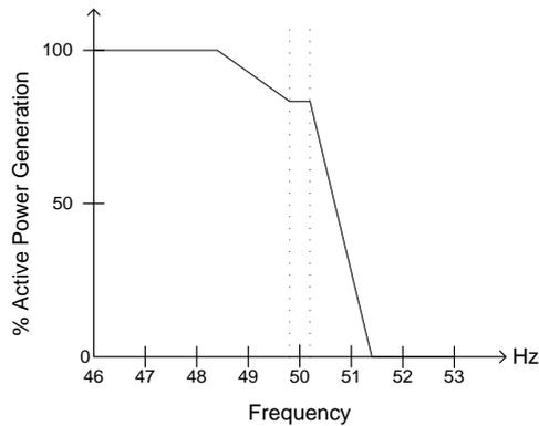
Figure 1: Power-frequency characteristic curve
