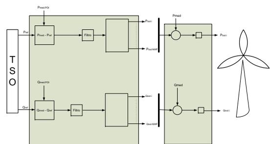
Figure 2: Hierarchical sketch for Wind Farm control
