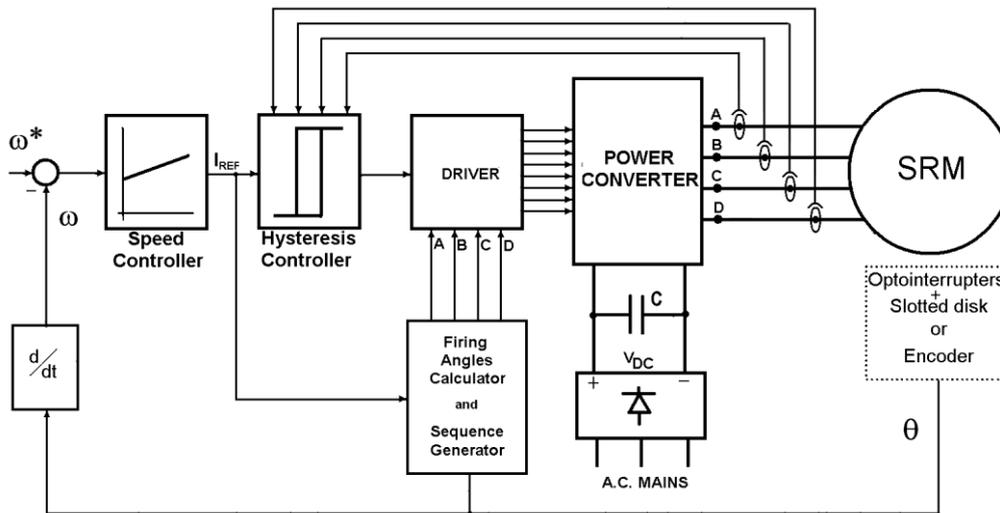
**Fig. 3.** Schematic diagram of the SRM drive
