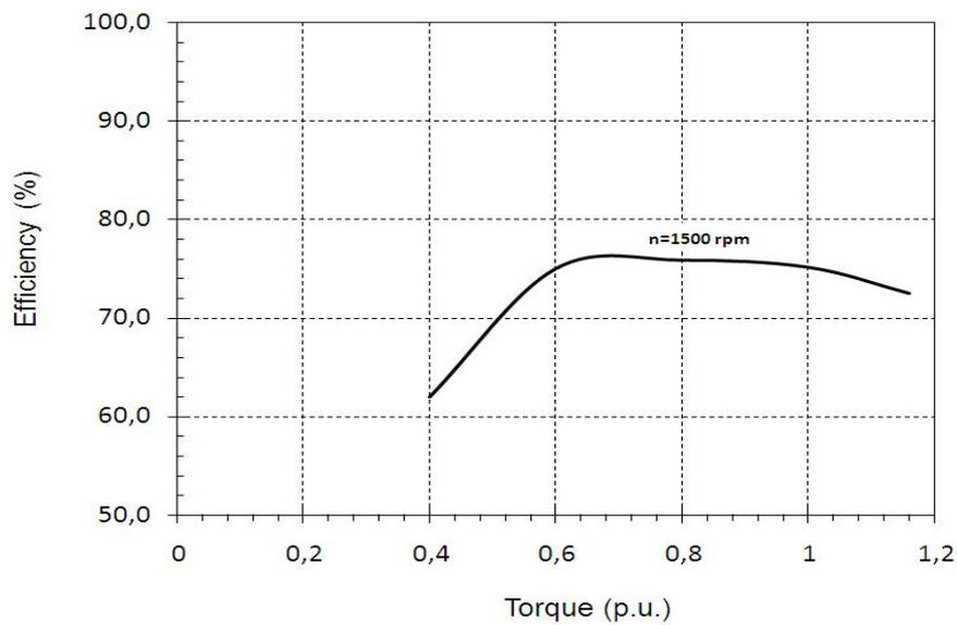
Fig. 4. Global efficiency vs. torque for the IM (Eff3) drive
