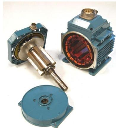
Fig. 1. Photograph of the disassembled 8/6 SRM
