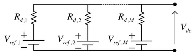
Fig. 5. Steady state model of parallel connected VSC DCVRs
