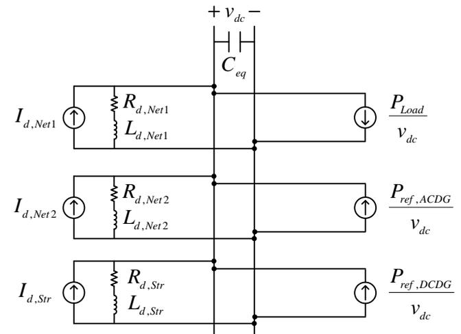
Fig. 10. Proposed large signal model of DCμG
