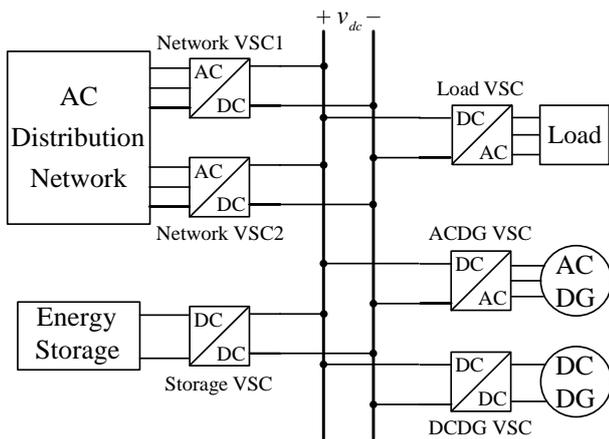
Fig. 1. General structure of DC $\mu$ G
