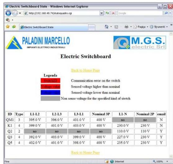
Fig. 8. Example of an on-line monitoring page
